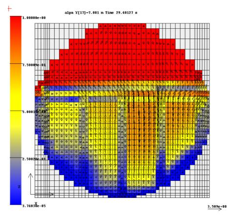
**Figure 7**: Colored map of void fraction and arrows of steam velocity component is for the SG middle section between "hot" and "cold" collectors. Velocity scale arrow in m/s is below write under map.
