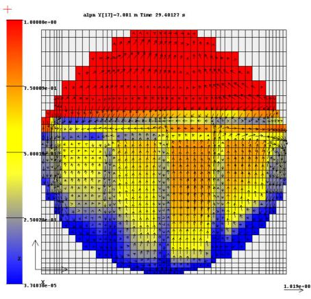
**Figure 6**: Colored map of void fraction and arrows of liquid velocity component is for the SG middle section between "hot" and "cold" collectors. Velocity scale in m/s arrow is below write under map.
