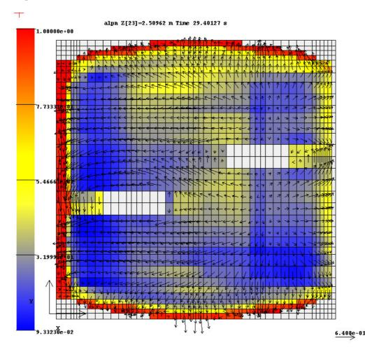
**Figure 8**: Color map of void fraction and arrows of liquid velocity component in m/s is shown for level of feed water distribution abovenag underwater porous plate. It is section with feed water collector position. Scaling arrow for liquid velocity is shown in bottom right.
