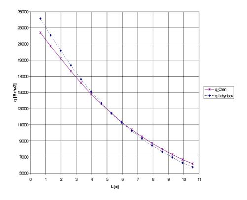
**Figure 9**: Comparison of calculation profiles of specific heat flux (on external surface of a tube) in function along length of tubes from "hot" to "cold" collectors for two versions. Versions:
