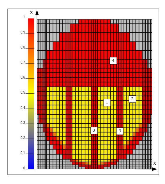
**Figure 3**: Calculation diagram of SG vessel in plane X-Z. Section Y=7,0 м (section between collectors). 1-Central packet. 2-Peripheral packet. 3-Corridors. 4- Gas volume. Volumetric coefficient of porosity is shown by color
