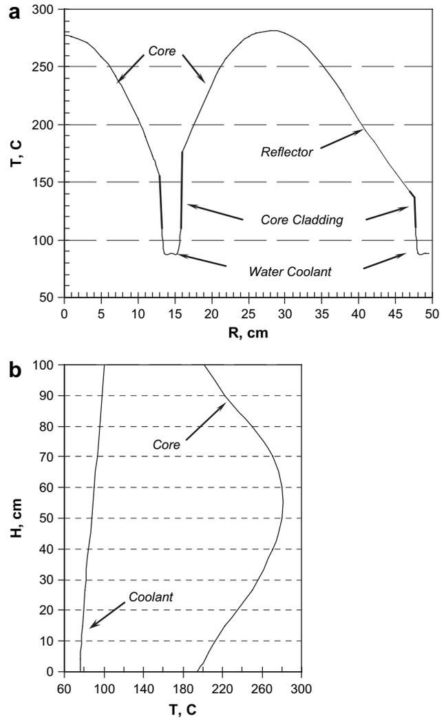
Fig. 3. Radial (a) and axial (b) core temperature distribution.
