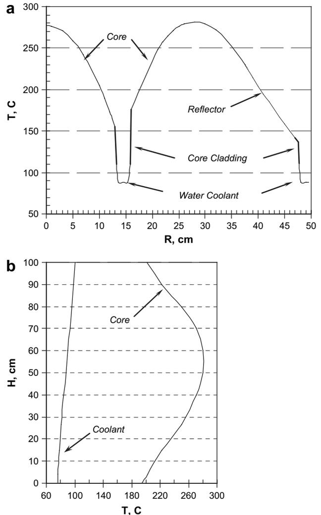
Fig. 3. Radial (a) and axial (b) core temperature distribution.
