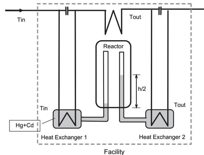
Fig. 6. Diagram of power self-control provided by inlet and outlet temperature of the consumer circuit.
