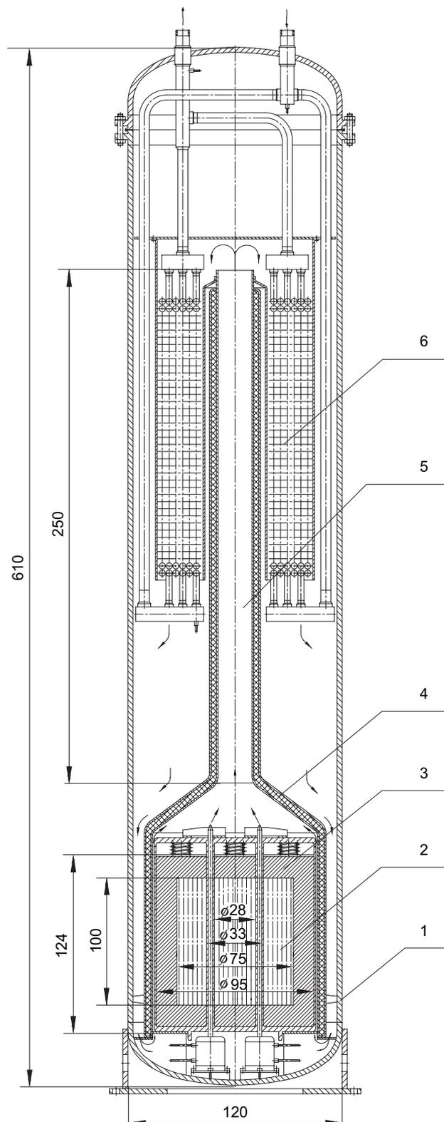
Fig. 2. Design diagram of the reactor facility MASTER (Dimensions are given in cm). 1, reactor vessel; 2, core; 3, reflector; 4, heat insulating shell; 5, draft tube; 6, heat exchanger.
