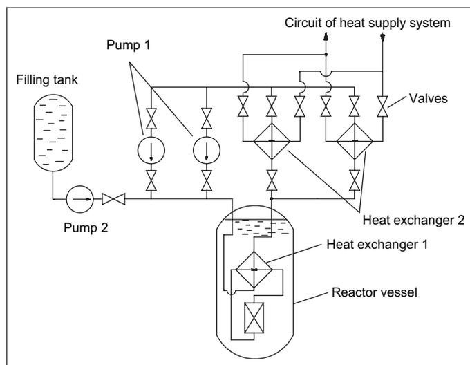
Fig. 1. Schematic hydraulic diagram of the reactor facility MASTER.
