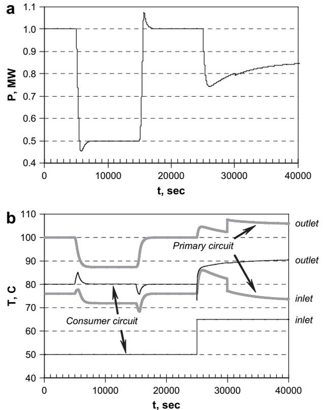
Fig. 7. Reactor power time behavior (a) and coolant temperature variations in the primary and consumer circuits (b) at the different perturbations.
