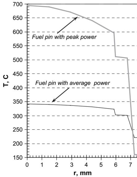
Fig. 4. Radial temperature distributions of the fuel pin for the average and for peak power.
