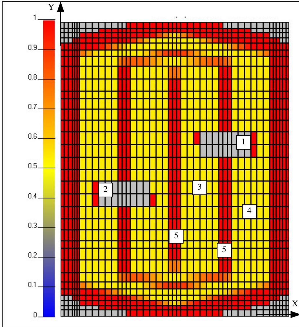
**Figure 2:** Calculation diagram of SG vessel in plane X-Y. Section at mark Z=2,19 m (section of top level of tube bundles). 1-Hot header. 2-Cold header. 3- Central packet. 4-Peripheral packet. 5-Corridors. Volumetric coefficient of porosity is shown by color.
