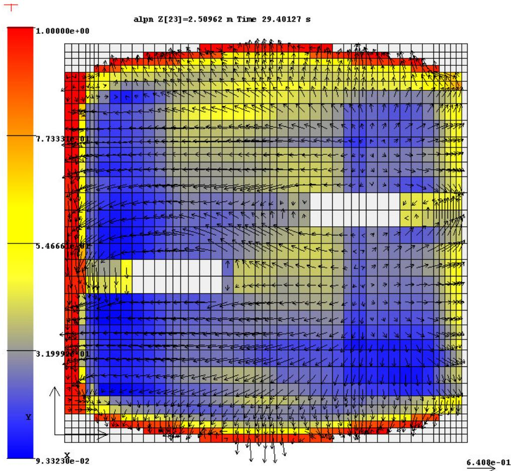
**Figure 8:** Color map of void fraction and arrows of liquid velocity component in m/s is shown for level of feed water distribution above underwater porous plate. It is section with feed water collector position. Scaling arrow for liquid velocity is shown in bottom right.
