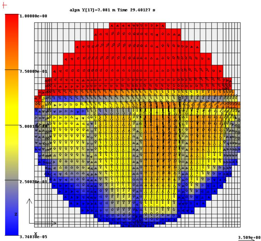
**Figure 7:** Colored map of void fraction and arrows of steam velocity component is for the SG middle section between “hot” and “cold” collectors. Velocity scale arrow in m/s is below write under map.
