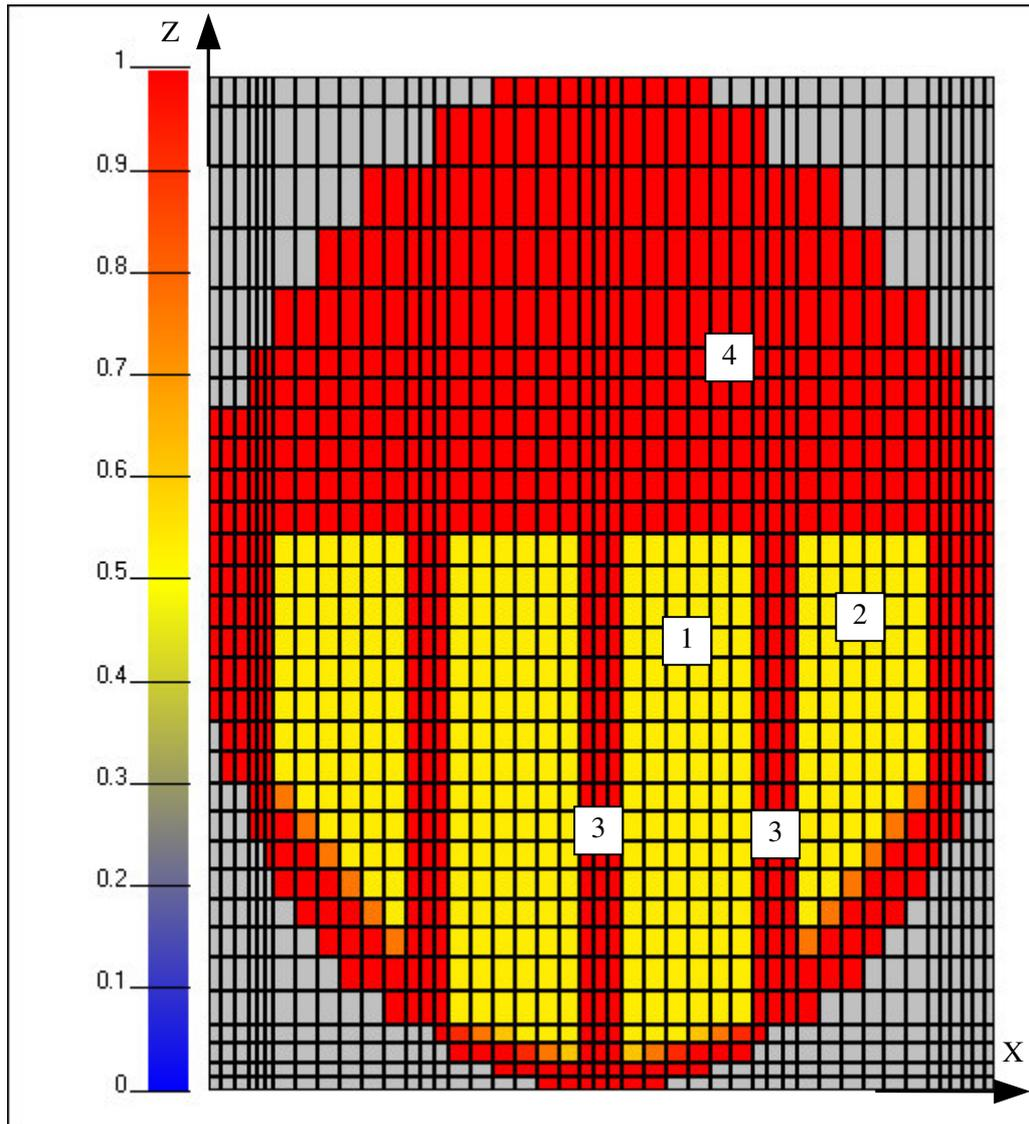
**Figure 3:** Calculation diagram of SG vessel in plane X-Z. Section  $Y=7,0$  m (section between collectors). 1- Central packet. 2-Peripheral packet. 3-Corridors. 4- Gas volume. Volumetric coefficient of porosity is shown by color
