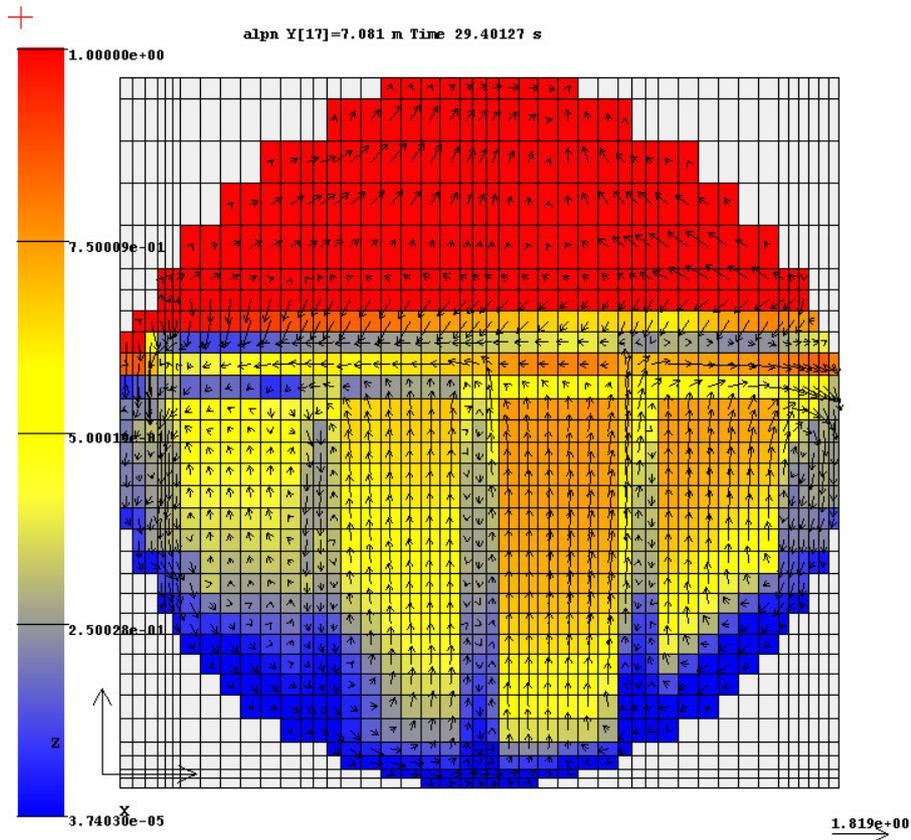
**Figure 6:** Colored map of void fraction and arrows of liquid velocity component is for the SG middle section between “hot” and “cold” collectors. Velocity scale in m/s arrow is below write under map.
