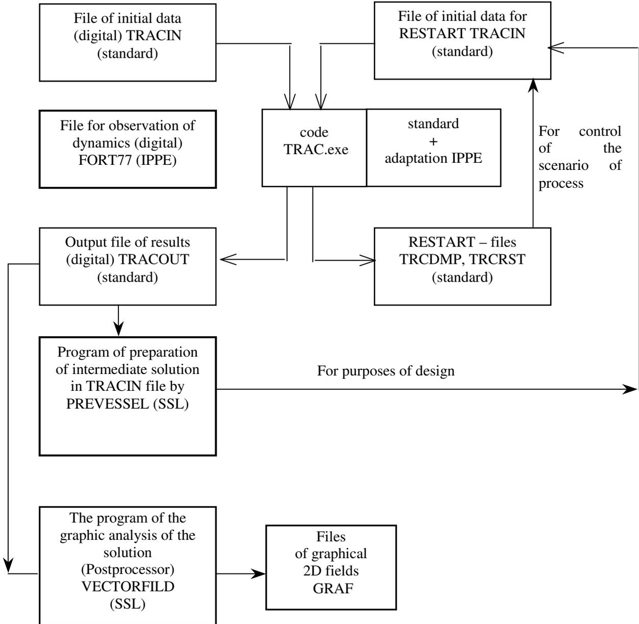
**Figure 5:** Block-diagram of the computer complex of programs
