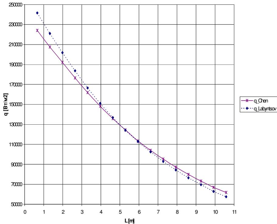
**Figure 9:** Comparison of calculation profiles of specific heat flux (on external surface of a tube) in function along length of tubes from “hot” to “cold” collectors for two versions.
