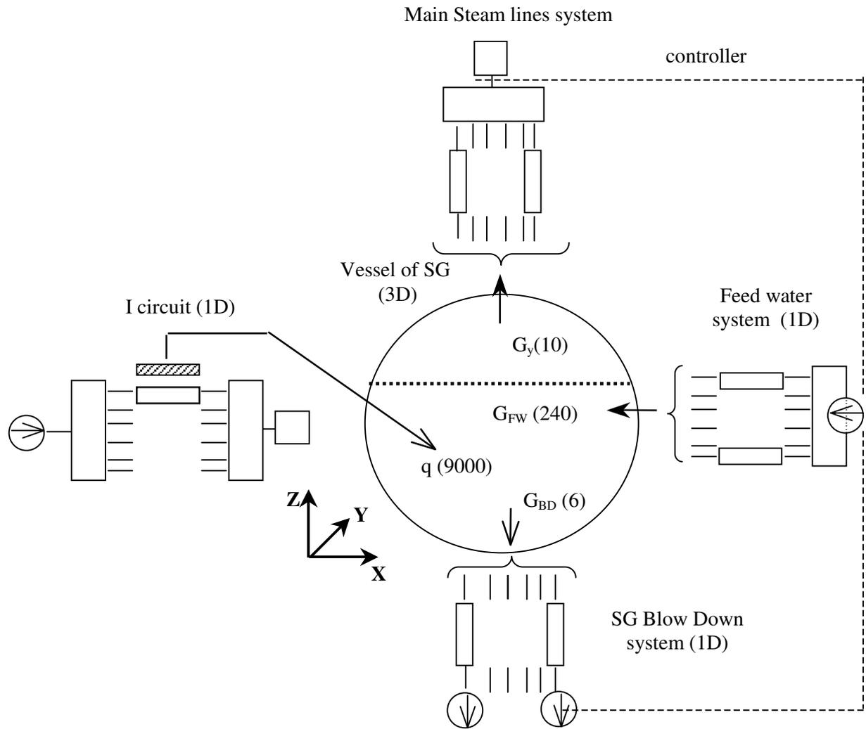
**Figure 1:** Calculation scheme of steam generator PGV-1000M.
